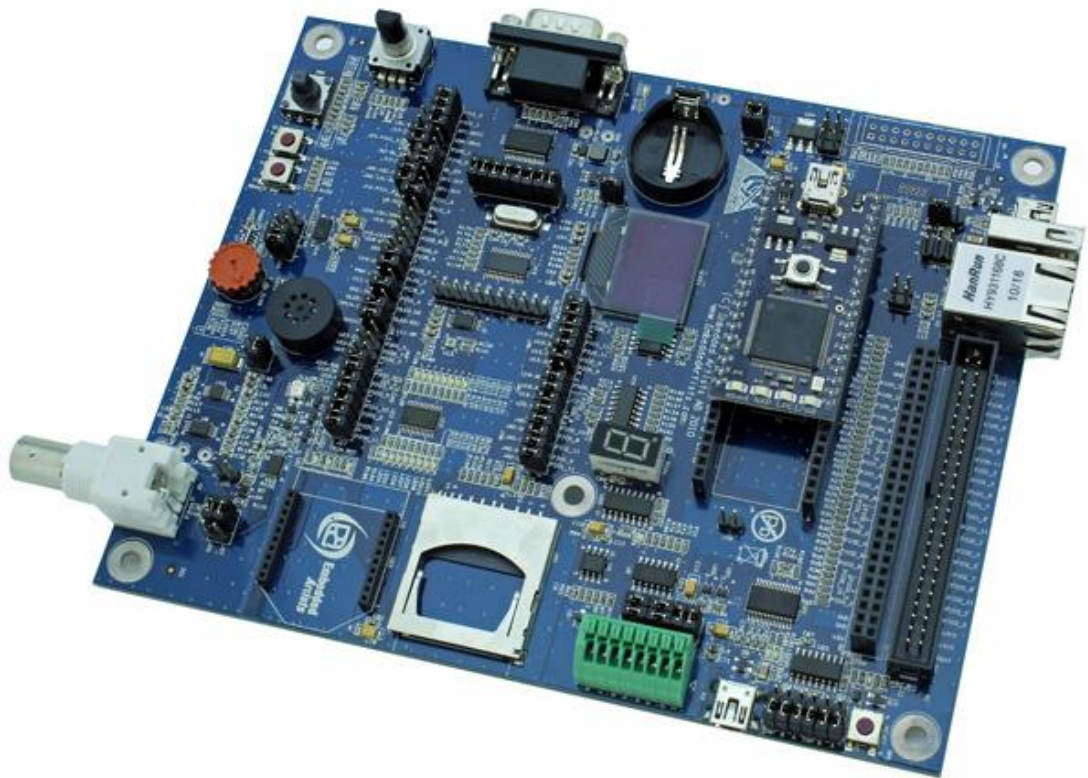
Figure 53 – mbed module mounted on LPCXpresso Base Board
