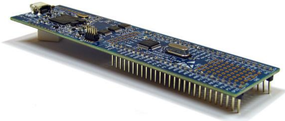
Figure 2 – LPCXpresso LPC1343 with pin list
